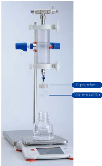
Virus Removal Filterability Testing Device
